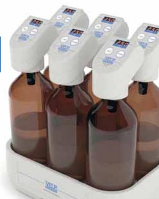
Perform your Biochemical Oxygen Demand analysis without altering the incubation condition. Manage up to 80 BOD sensors directly from your PC thanks to the unique connectivity of VELP BOD EVO.
